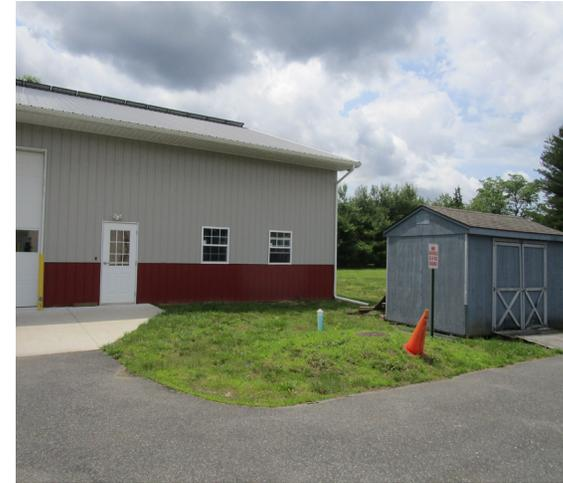
A rain garden can be installed on the west side of the building to manage stormwater runoff from the roof. A rainwater harvesting system can be installed at three corners of the shed to collect stormwater runoff from the roof. This can be used to clean fire trucks and for other non-potable purposes. A preliminary soil assessment suggests that the soils have suitable drainage characteristics for green infrastructure.
