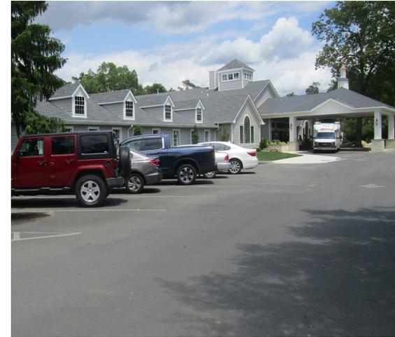
A rain garden can be installed near the entrance to manage rooftop runoff and create wildlife habitat. Parking spaces near the entrance can be converted to porous pavement to collect and infiltrate stormwater runoff from the roof as well. A preliminary soil assessment suggests that more soil testing would be required before determining the soil's suitability for green infrastructure.
