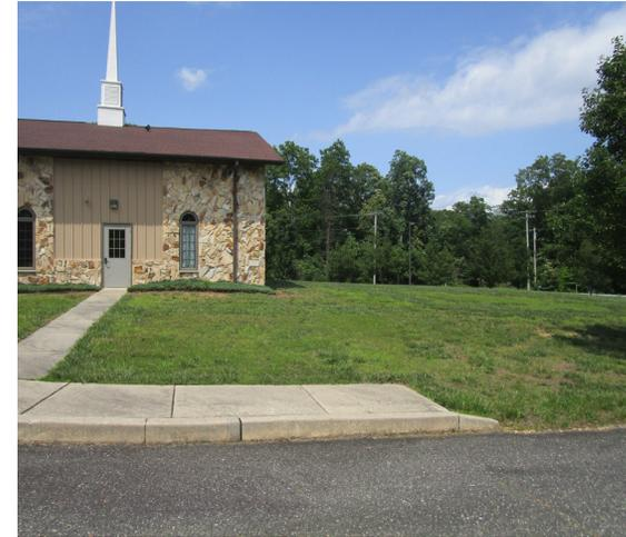
A rain garden can be installed on the east side of the building to manage stormwater by collecting rainwater from the roof. Rain gardens also provide aesthetic value and create wildlife habitat while managing stormwater runoff. Porous pavement can be installed to collect and filter stormwater on the west side of the building. A preliminary soil assessment suggests that more soil testing would be required before determining the soil's suitability for green infrastructure.
